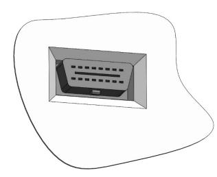
• remove the original OBD socket jack from it's housing (it's often times located behind the plastic panel)
